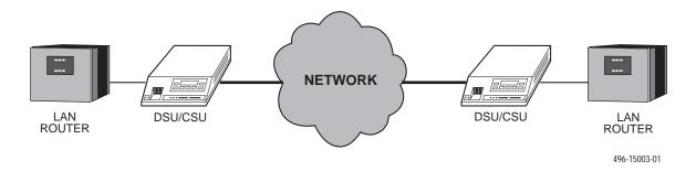
Figure 2-1. Point-to-Point Application Example
